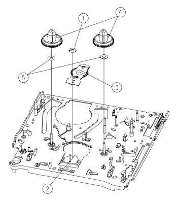
Fig.3-19 IDLER PLATE TOTAL ASS'Y & S/T REEL TABLES REMOVAL
